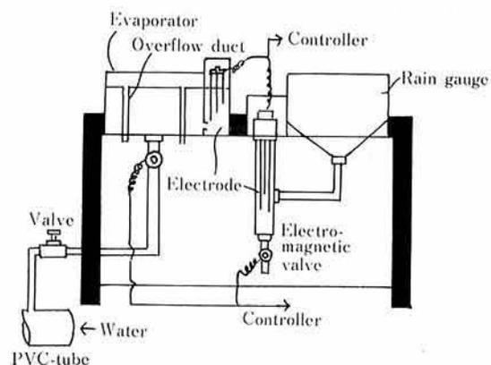
Fig. 3. Apparatus for automatic control of irrigation
