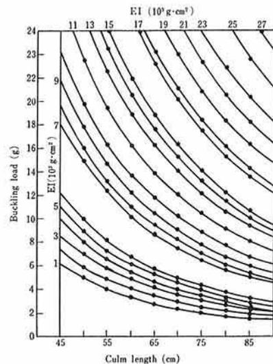
Fig. 2. Interrelation of buckling load and culm length.
