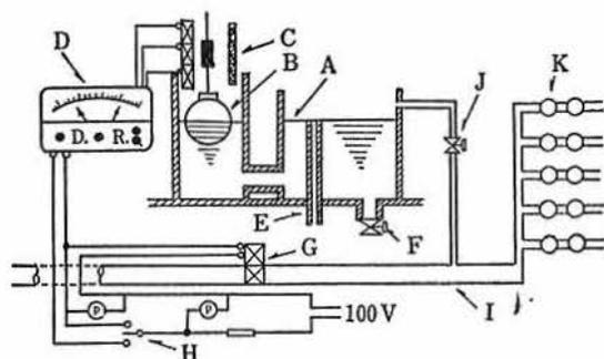
Fig. 6. Construction details of a new automatic irrigator
