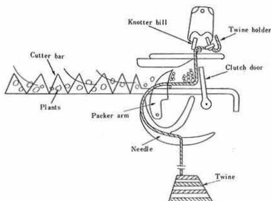
Fig. 3. Binding apparatus
