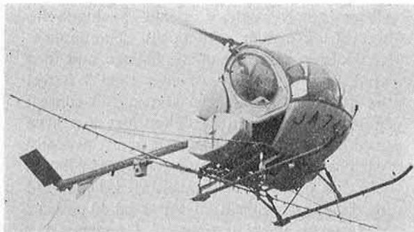
Fig. 5 Liquid application Kit of Helicopter
