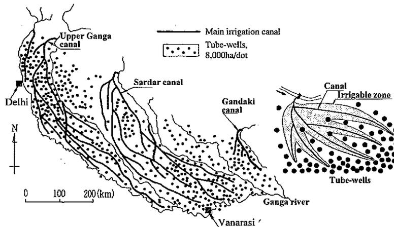
Fig. 12 Combined use of canals and groundwater in northern Indian plains Water distributed to a large region by the giant canal networks is actually used at field level through SDWs (shallow dug-well) or STWs (shallow tube-well) sunk in the individual farms.
