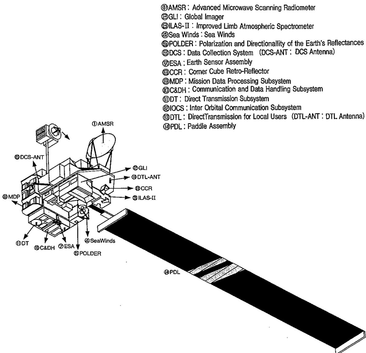
Fig. 2 Illustration of the ADEOS-II satellite and its five sensors
