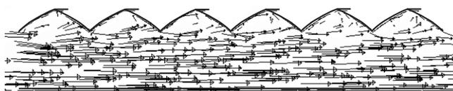
**Fig. 7. The effect of side vent opening on the airflow pattern in a 6-span greenhouse**
