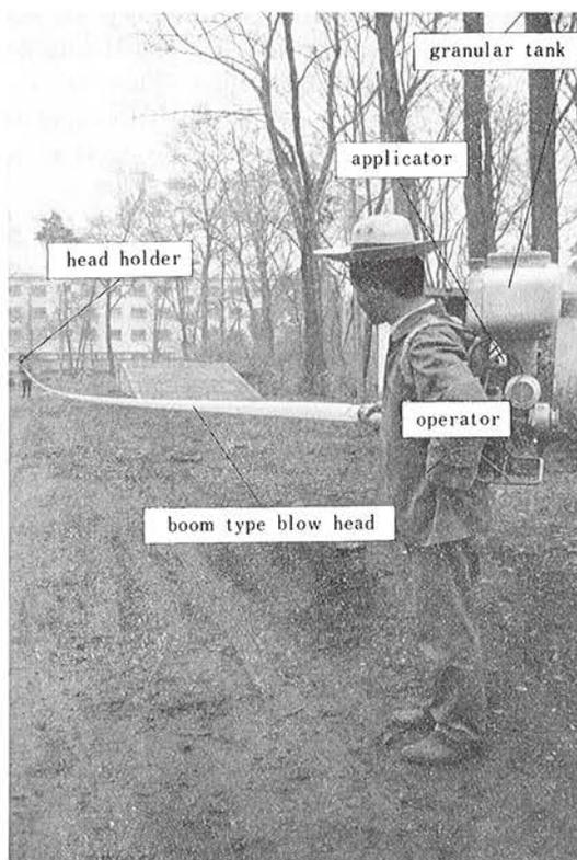
Fig. 1. Knapsack type power granular applicator
