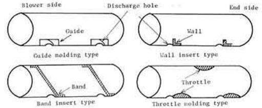
Fig. 2. Granular boom type blow head
