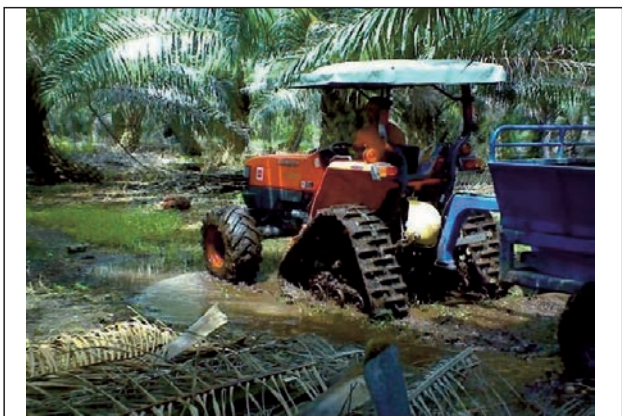
Crawler Tractors (28 - 45 hp) suitable for FFB evacuation in soggy area in oil plantation, Malaysia
