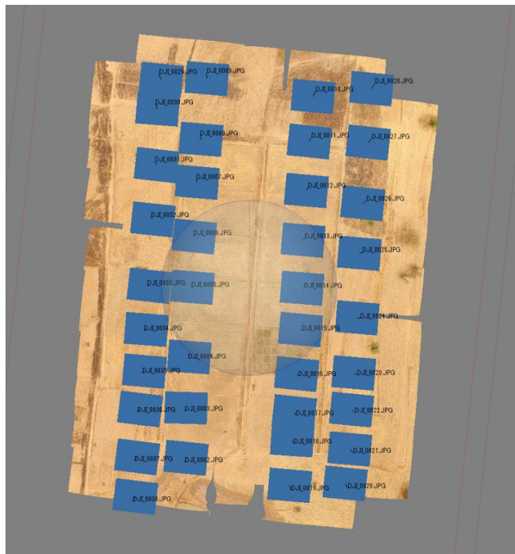
Fig.1.13 Photographic points for the field at Nwogu village
