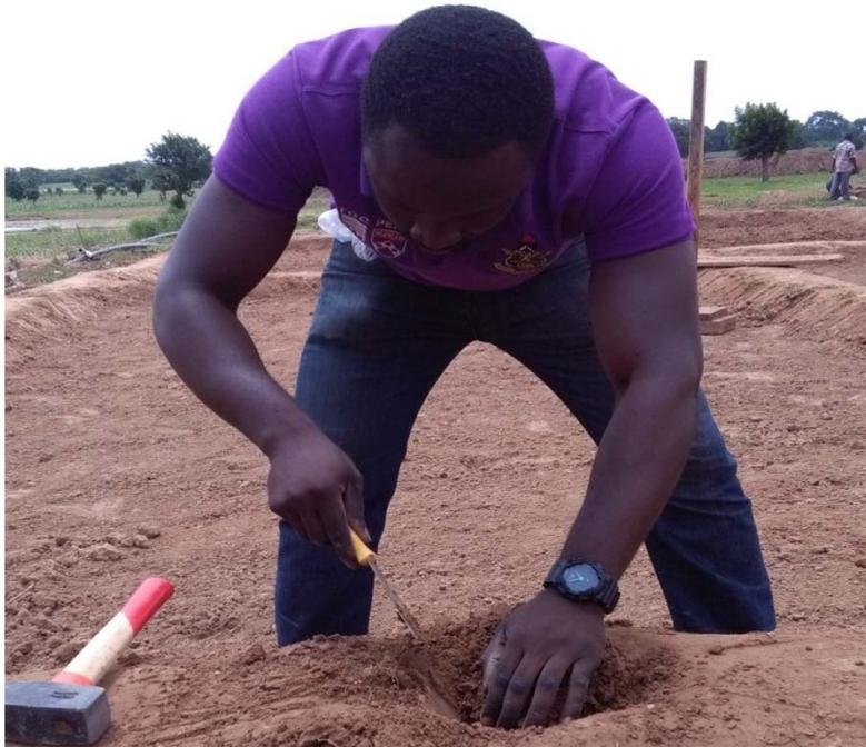
Fig. 2.42 Taking soil sample
