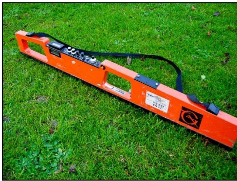
Fig. 3.1.2 EM38 Ground Conductivity Meter
