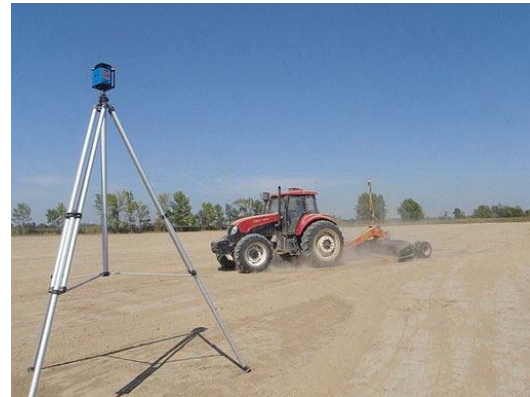
Fig. 2.1.13 Laser land leveling
