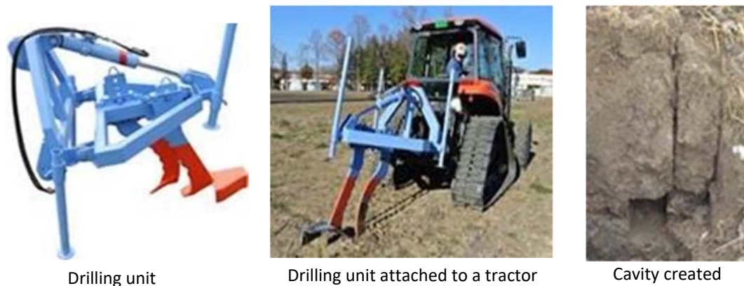
Fig. 4.1.2 The drilling unit and a cut-drain
