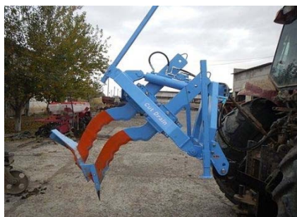
Fig. 4.3.9 Blade position during relocation
