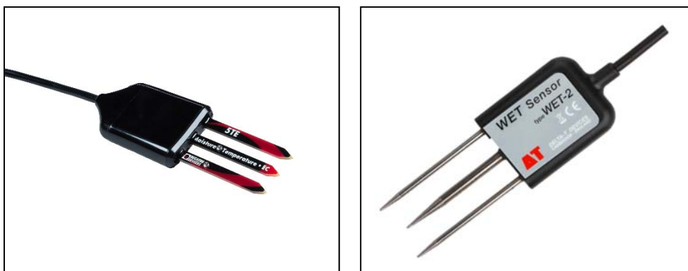
Fig. 3.1.1 Soil moisture, EC sensor (left: 5TE, right: WET2)
