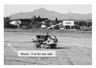
Fig. 7. Variable rate granular fertilizer applicator with a GPS and 10 m boom for applying coated urea as a basal nitrogen fertilizer
