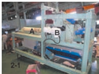
Fig.2. The shredder which crushed the inner parts of palm trunks (palm trunk core) into small chips (2-1), and the press mill which squeezed sap from the small chips (2-2).
