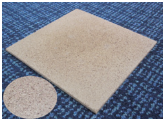
Fig. 1. Binderless particleboard made from oil palm trunk. Inset shows the magnified image of the surface.
