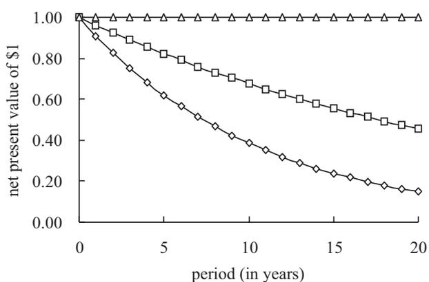
Fig. 5. Net present value with different discount rates
